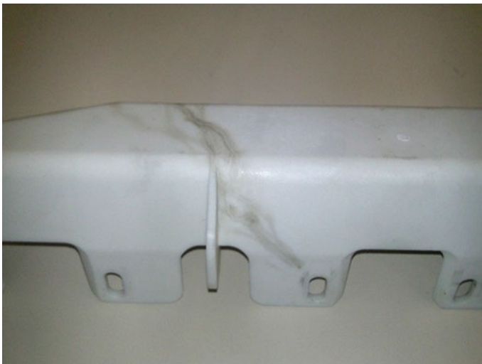
Fig. 4 Traces of flashover on the surface of a thermoplastic part
