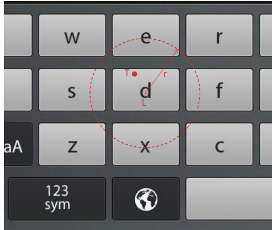
Fig. 2. Computing the distance based score for a given letter, “d”. The position of the letter “d” is denoted L, the actual touch location, T, and the radius of circle, r. Outside the circle the normalized distance is clamped to 1, otherwise, (T-L)/r .
