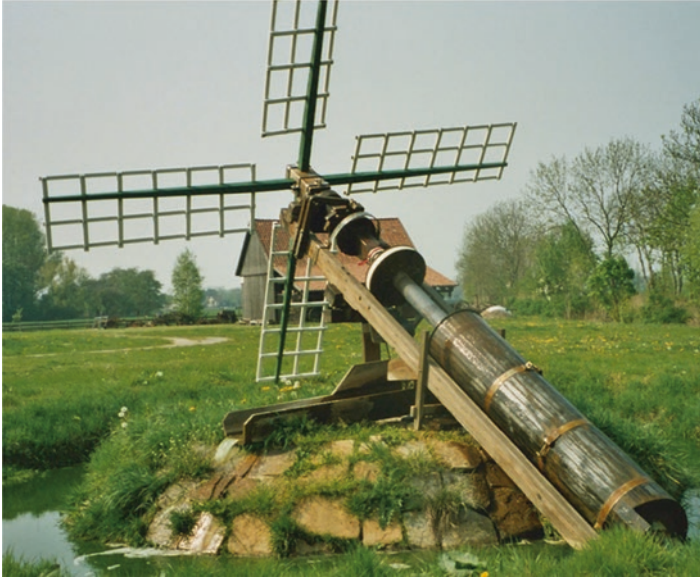
Figure 4 Flutter-Mill: Moorseer Windmill in Weser-Marsh, Germany, for the drainage of marsh land. Such wind-powered screws were also used for salt making (as in Spain)
