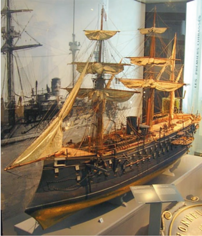
Figure 13 The ram is introduced to iron warships: French ironclad Solferino , 1861
