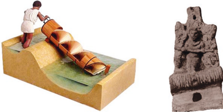
Figure 1 (left) Modern depiction of an Archimedes screw turned by a farmer. (right) Egyptian terracotta figurine (about 30 BC)
