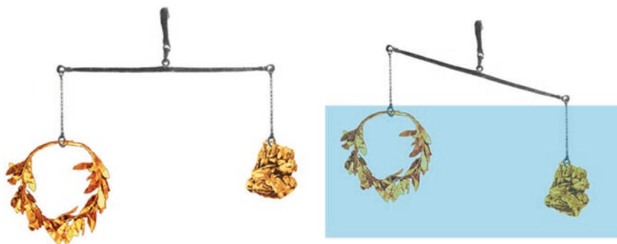
Figure 16 Crown and gold nugget—balanced in air ( left ), but unbalanced in water ( right )
