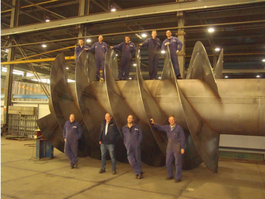
Figure 10 Hydropower screw manufactured by Landustrie in the Netherlands ( D_a = 4.5 meters)
