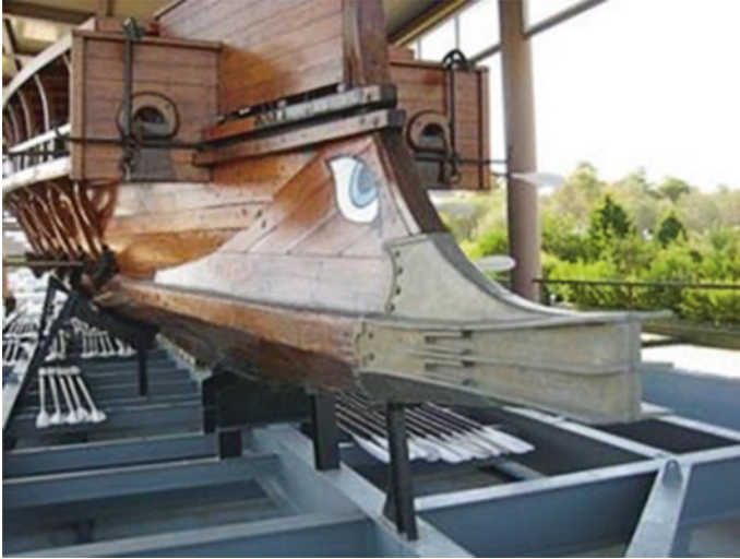
Figure 8 Ram bow of Olympias , a modern replica of a Greek trireme
