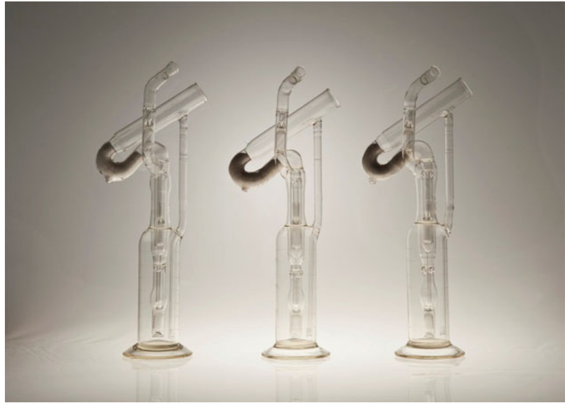
Fig. 4 The Glass Heart in the National Museum of American History. This is the device Carrel and Lindbergh used to maintain whole organs for days at a time to study function in isolated culture. (Reproduced from the NMAH website https://americanhistory.si.edu/collections/search/object/nmah_688713 )
