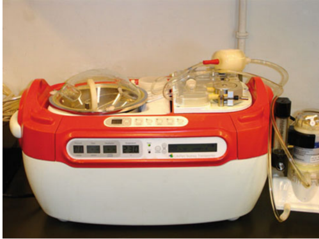
Fig. 3 Portable perfusion pump. The HeartPort© System is a modified version of the LifePort© System (Organ Recovery Systems©, Itasca, IL, USA), designed for kidney graft perfusion and preservation. The heart grafts were suspended inside a sterile cassette and subjected to retrograde perfusion with 1 L asanguineous preservation
