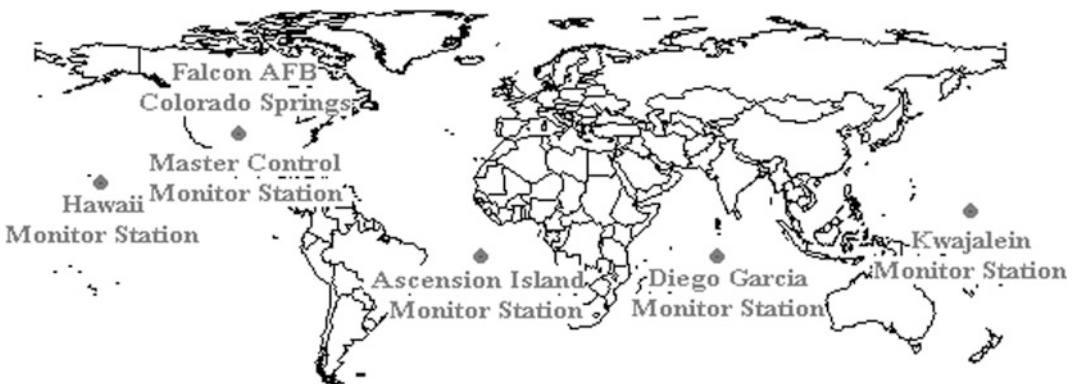
Fig. 4.2 Master control and monitor station of NAVSTAR
