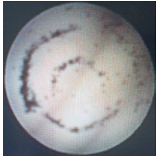
Fig. 3.6 Black dots corresponding to broken fibers after the ultrathin fibrobronchoscope was accidentally bitten by a patient
