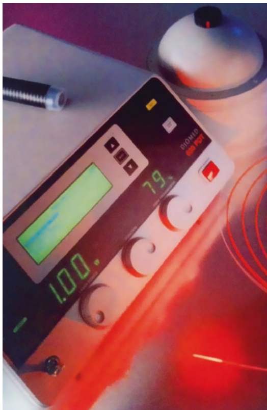
Fig. 11.2 Diode laser of 630 nm
