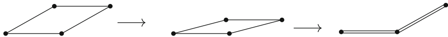
Fig. 7.10 An invariant cyclic graph of order 4 has geometric spectrum corresponding to realizations in the plane as a polygonal framework with sides of equal length
