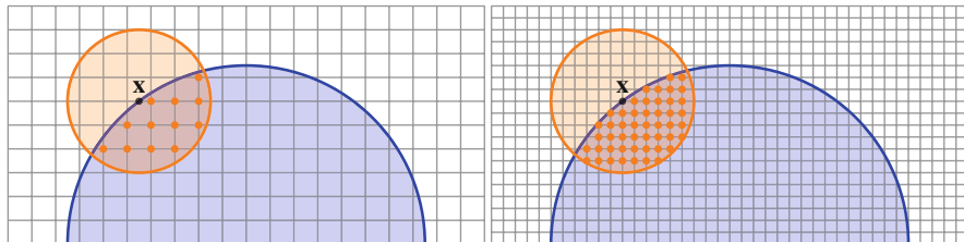
Fig. 9.3 Illustration of 2D integral digital curvature estimator \hat{\kappa}^R . The shape X is a disk of radius 7.5. To the left, the digitization gridstep h is 1, while h is 0.5 to the right. We choose a ball of radius R = 3 and we wish to estimate the curvature at some arbitrary point \mathbf{x} . We count the number of digital points within the orange ball, centered at \mathbf{x} and of radius 3. To the left we count 12 points. Hence for h = 1 , the estimated curvature \hat{\kappa}^3(G_1(X), \mathbf{x}, 1) is 3\pi/(2 \times 3) - 3 \times 12 \times 1^2/3^3 \approx 0.237 . To the right we count 50 points. Hence for h = 0.5 , the estimated curvature \hat{\kappa}^3(G_{0.5}(X), \mathbf{x}, 0.5) is 3\pi/(2 \times 3) - 3 \times 51 \times 0.5^2/3^3 \approx 0.154 . Ground truth curvature is 1/7.5 \approx 0.133
