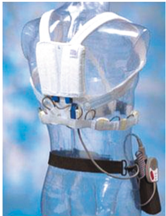
Fig. 11.6 This figure shows the wearable defibrillator (LifeVest) which consists of straps, holding non-adhesive sensing electrodes and dry shocking electrodes that release conductive gel prior to shock delivery. The monitor is worn on the waist. In the event of arrhythmia detection, it will provide auditory, visual, and tactile alarms. If conscious, the patient can press two buttons simultaneously to prevent a shock
