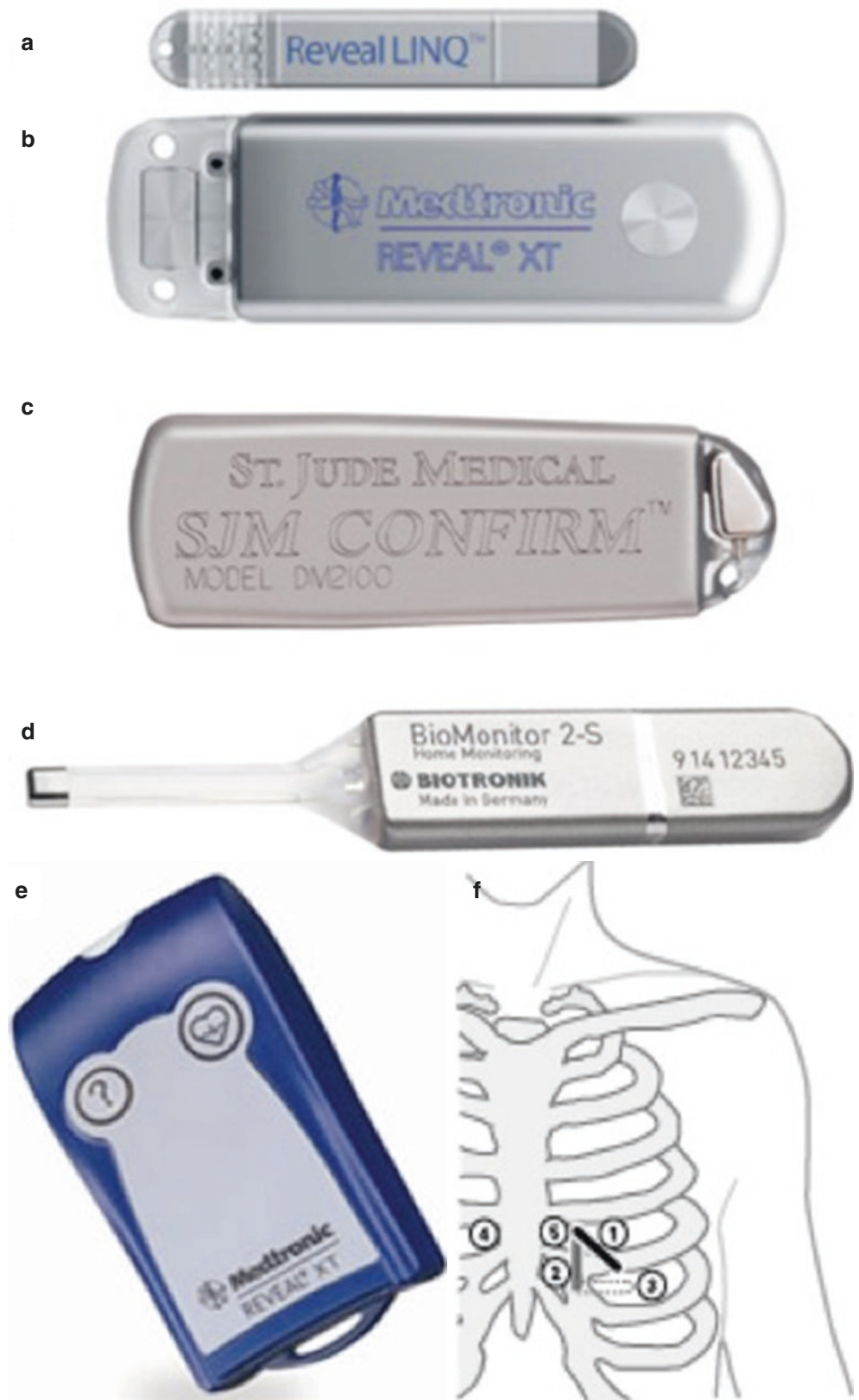
Fig. 5.4 Examples of commonly used ICMs. (a) Medtronic Reveal LINQ™ (Medtronic, Minneapolis, MN, USA). (b) Medtronic REVEAL XT® 9529 (Medtronic, Minneapolis, MN, USA). (c) St. Jude Medical™ Confirm DM2100 (St. Jude Medical, St. Paul, MN, USA). (d) BioMonitor 2 (Biotronik, Berlin, Germany). (e) Patient assistant for all Medtronic ICMs. (f) Recommended insertion locations for Medtronic Reveal LINQ™. The preferred subcutaneous location is over the fourth intercostal space along the V2-V3 electrode orientation with a 45° angle to the sternum. Alternatively the device can be inserted over the fourth intercostal space, parallel to the sternum with a distance of 2 cm ± 1 cm
