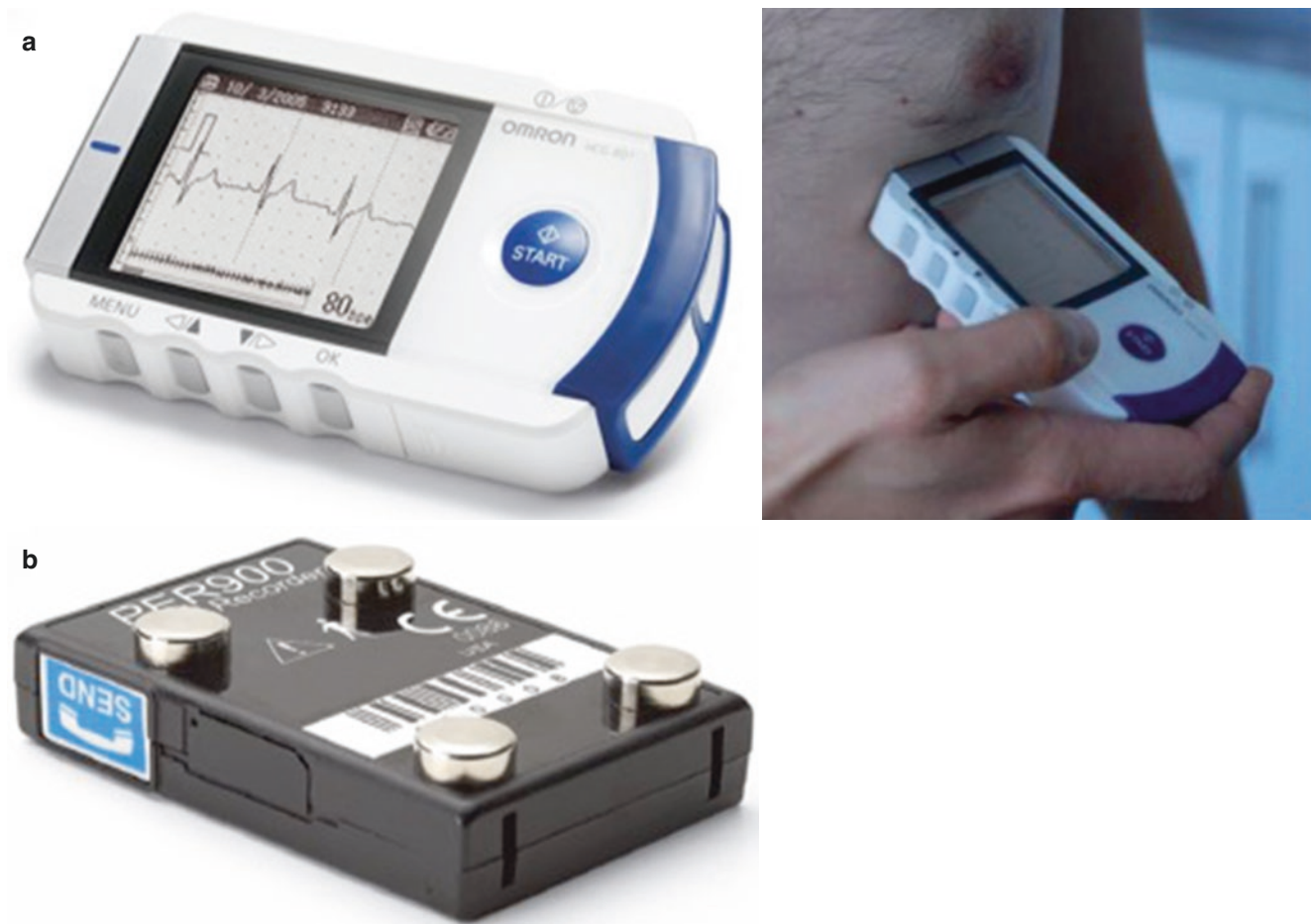
Fig. 5.2 Examples of non-looping (post event) external cardiac event recorders. (a) Omron HeartScan HCG-801® (Omron Healthcare, Kyoto, Japan). (b) Braemar PER900 Post Event™ (Braemar, Eagan, MN, USA)
