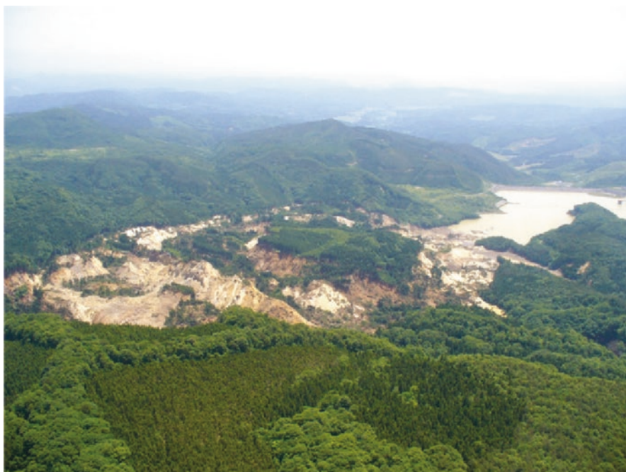
Fig. 10.5 Aratosawa landslide caused by earthquake (Length: 1.3 km, Width: 1 km, Volume: 6 million m 3 )
