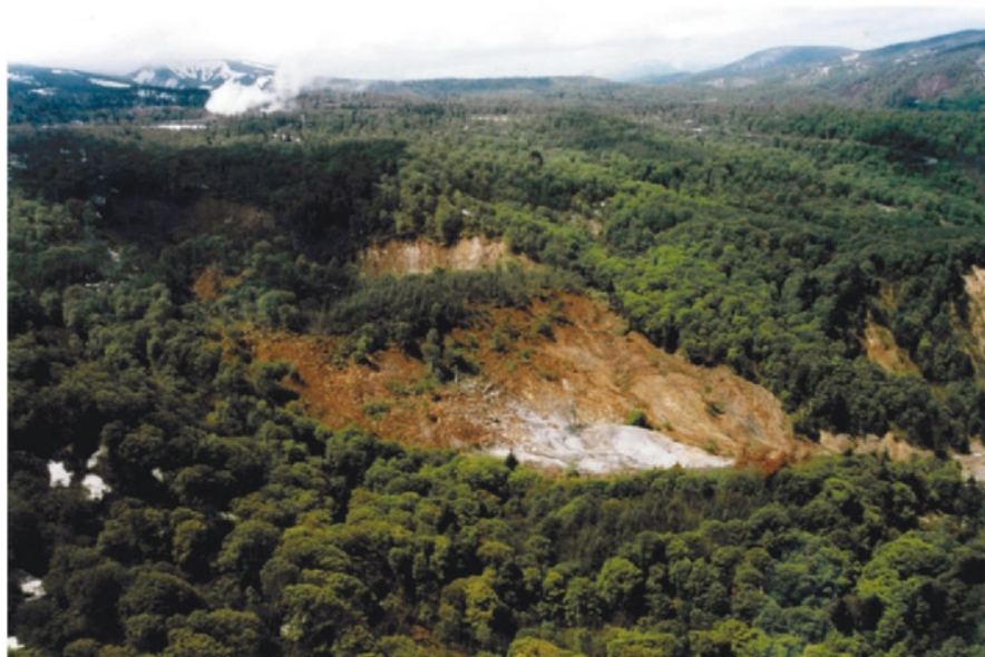
Fig. 10.4 Hachimantai landslide caused by snowmelt (Length: 700 m, Width: 400 m, Volume: 70 million m 3 )
