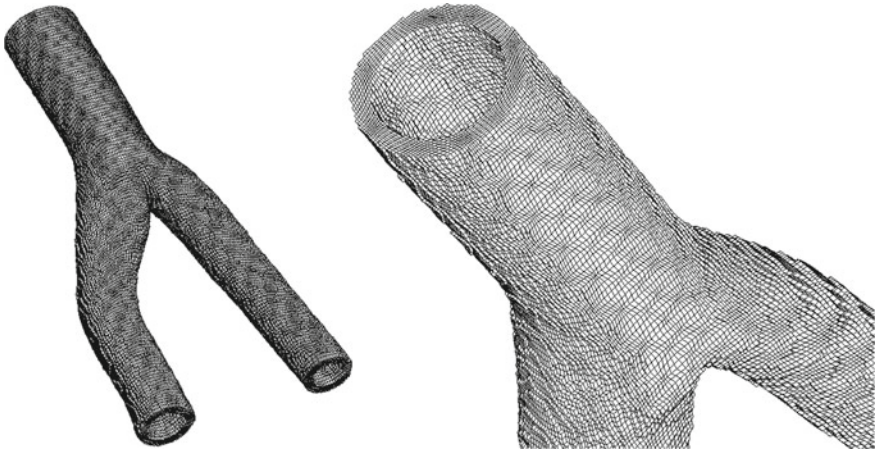
Fig. 13.31 Hexahedral mesh modelling the walls of an aorta and carotid arteries
