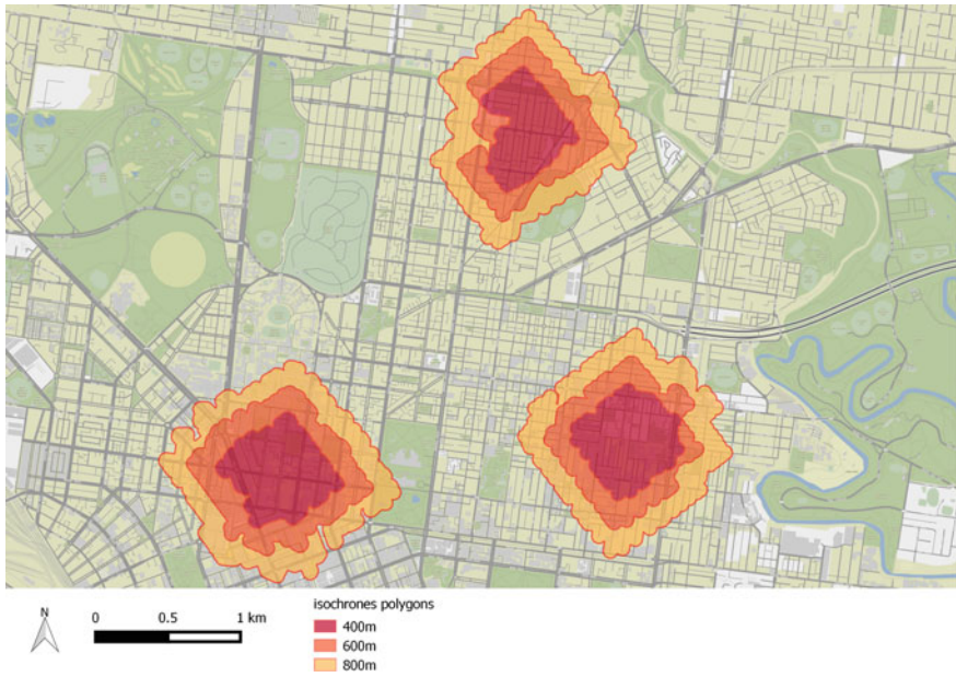
Fig. 8 Calculate isochrones for N points with various distances with combotype set to “ composite ” (by walk)
