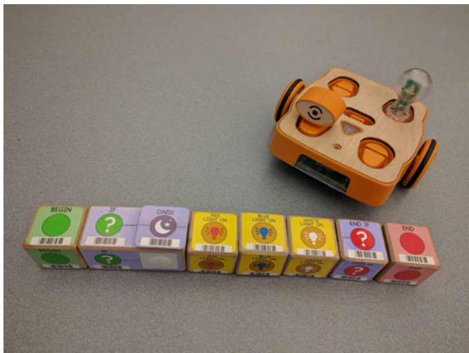
Fig. 10.20 Robot with light sensor and light output, and program to turn on lightbulb in the dark
