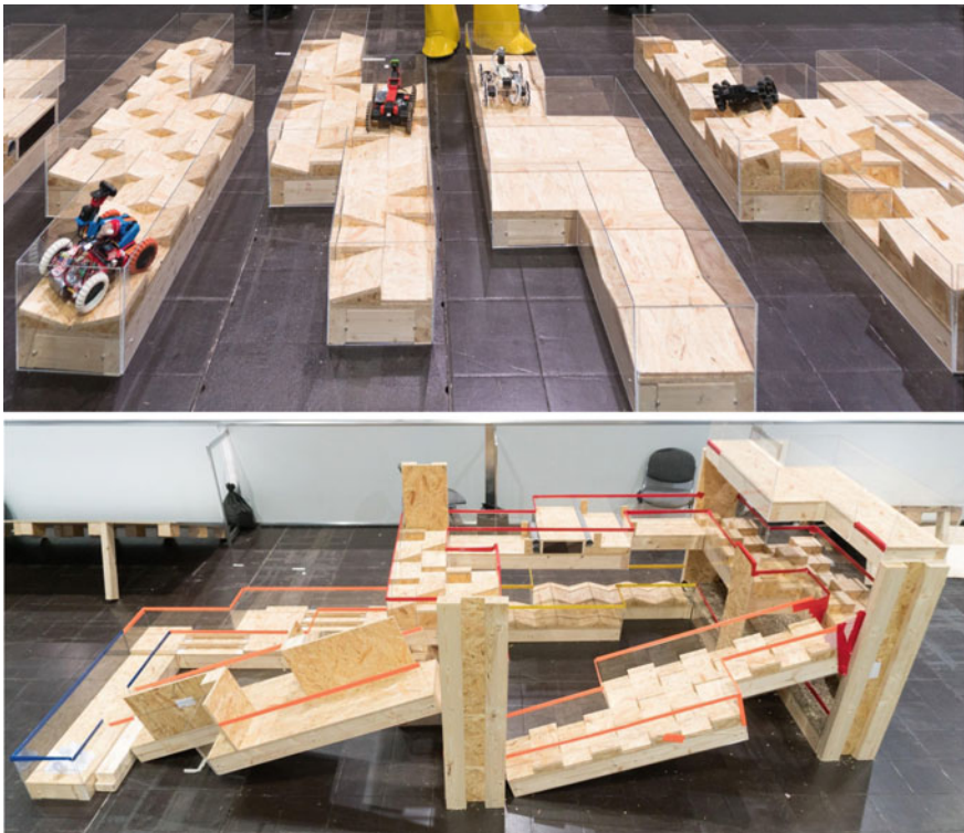
Fig. 4.5 Rapidly Manufactured Robot Competition arena as configured for the preliminary rounds ( top ) and the finals ( bottom )
