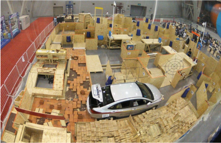
Fig. 4.3 The RRL arena. This is a test course for response robots of various shapes and sizes and is built based on a 1.2-m grid. An early version of the Rapidly Manufactured Robot Competition arena is visible embedded on the left
