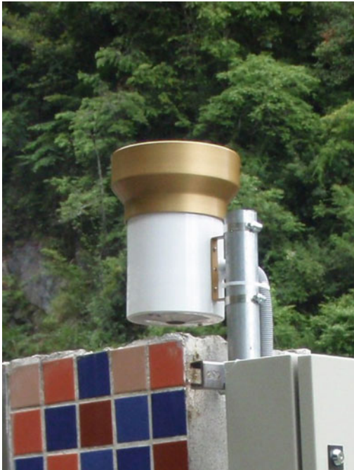
Fig. 6 A tipping bucket rain gauge (DECL, Taipei, Taiwan)
