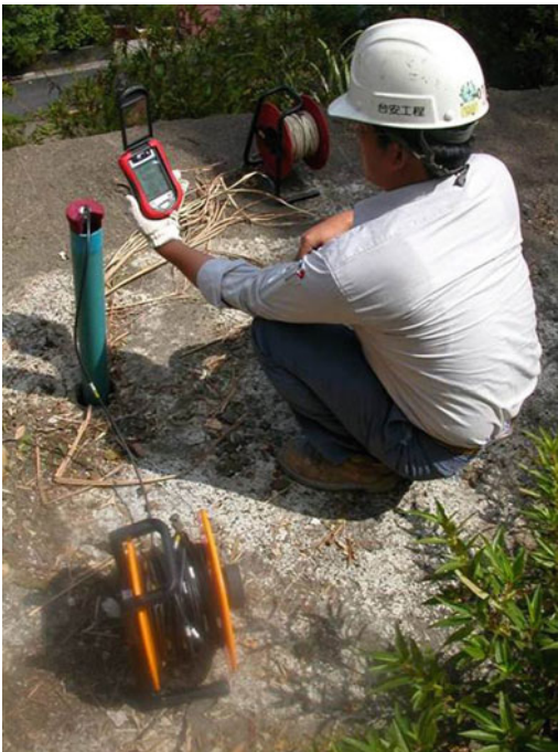
Fig. 4 Taking inclinometer probe readings in the field (DECL, Taipei, Taiwan)
