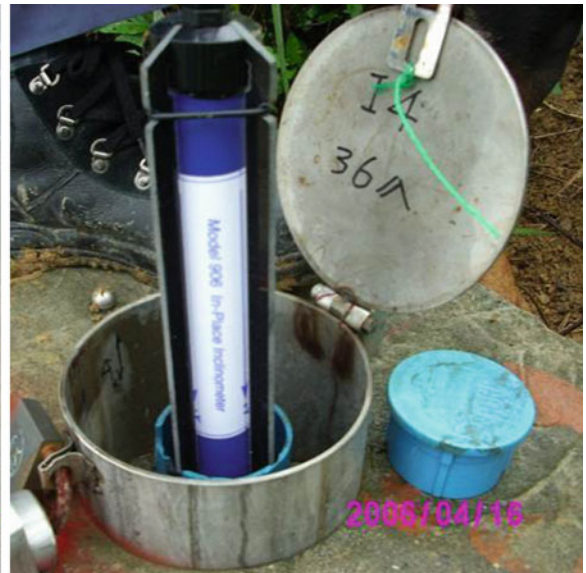
Fig. 10 Field installation of in-place inclinometers (DECL, Taipei, Taiwan)
