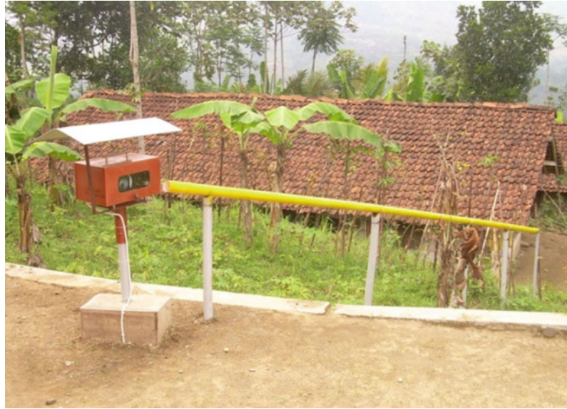
Fig. 3 Placement of an automatic extensometer
