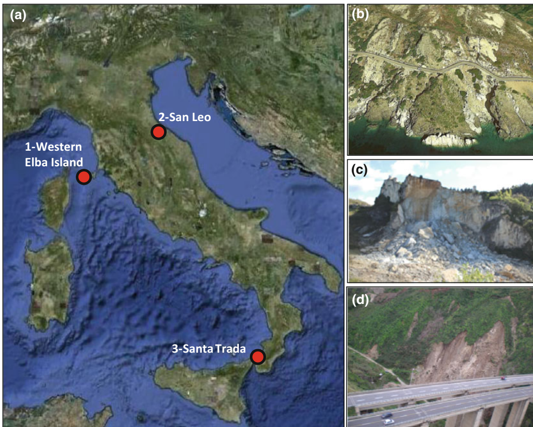
Fig. 3 a Case studies location; b Western Elba Island (unstable rock masses); c San Leo (collapsed rock cliff); d Santa Trada (planar slide in metamorphic weathered rocks)
