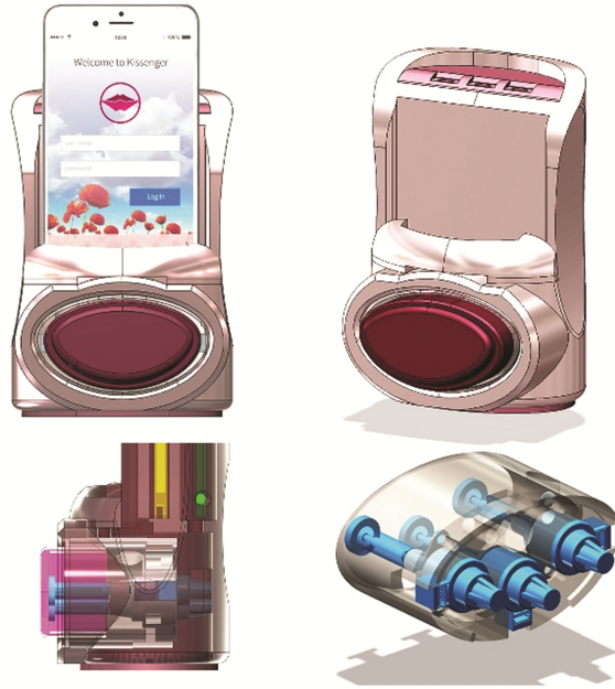
Fig. 7. 3D models of the Kissenger haptic interface in the form of a mobile phone case with additional actuators and sensors
