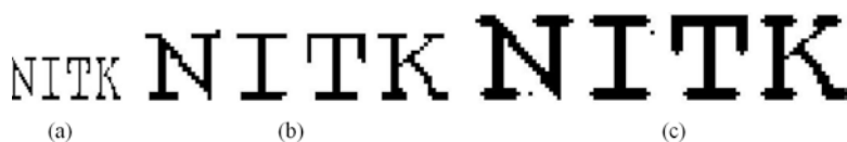
Fig. 6.4 Recovered watermark of different size at gain factor = 5 (a) 64 \times 20 ; (b) 80 \times 25 ; (c) 99 \times 31
