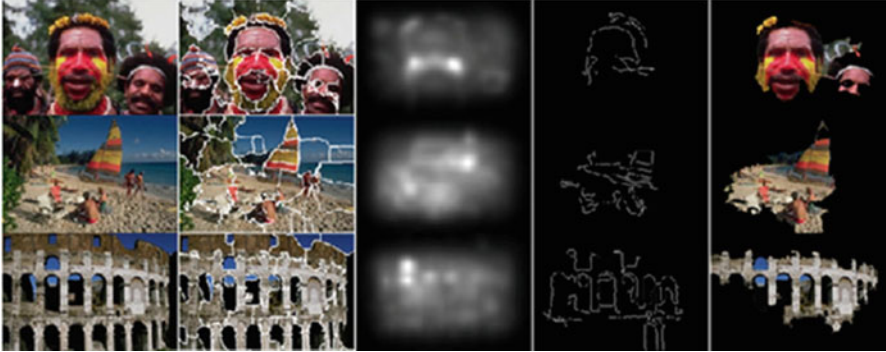
Fig. 11 Examples of extracted query information: (1) Original, (2) Image segments, (3) Saliency map, (4) Salient edges, (5) Selected salient regions
