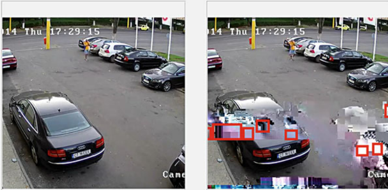
Fig. 6.10 In city-scale video processing, artifacts induced by spatial and temporal compression can severely impair the performance of detection and tracking algorithms
