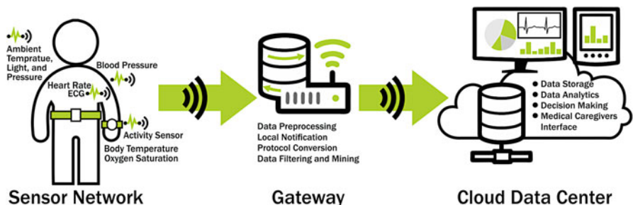
Fig. 8.4 Healthcare IoT system architecture
