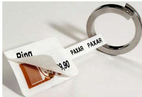
Fig. 5. A RFID with a chip storing a digital signature
