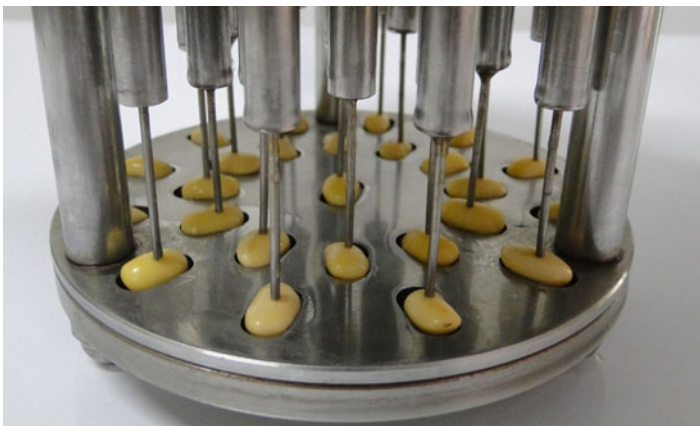
Fig. 20.1 Positioning of soybeans in the Mattson-type equipment. Uberaba, Minas Gerais. Photo: Juhász et al. 2014
