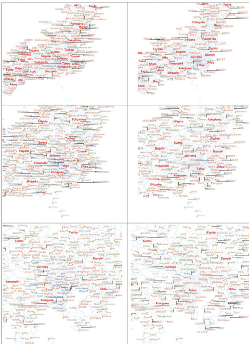
Fig. 5 Label placement around Tokyo, Japan. Left Naïve inconsistent placement. Right Scale-aware consistent placement. Different colors are assigned to the names according to their administrative levels; the prefecture, city, county, and town names are in red, orange, green, and gray, respectively
