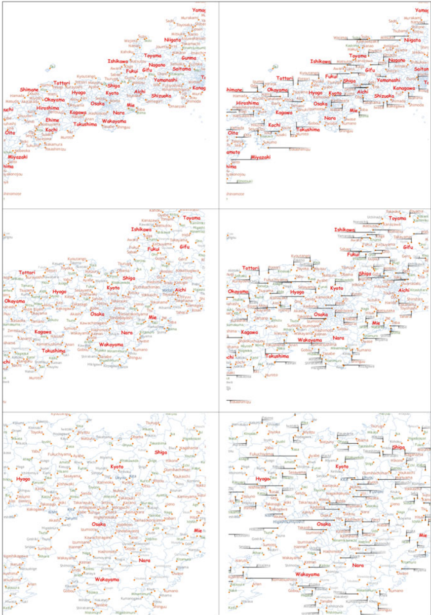
Fig. 6 Label placement around Osaka, Japan. Left Consistent placement with four label positions. Right Consistent placement with 16 label positions. Different colors are assigned to the names according to their administrative levels; the prefecture, city, county, and town names are in red , orange , green , and gray , respectively
