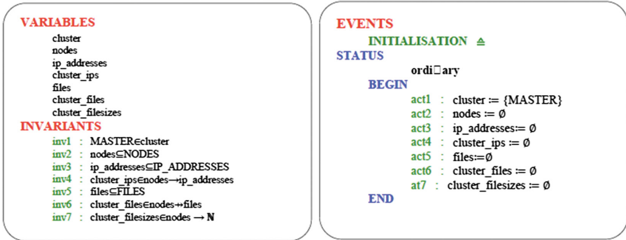
Fig. 8. (a) Variables and invariants of “Cluster_Mac0” (own work), (b) Initialization of “Cluster_Mac0” (own work)
