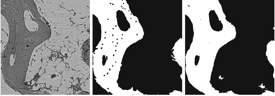
Fig. 6. Example results: original grayscale image (left), reference (middle), obtained segmentation (right)
