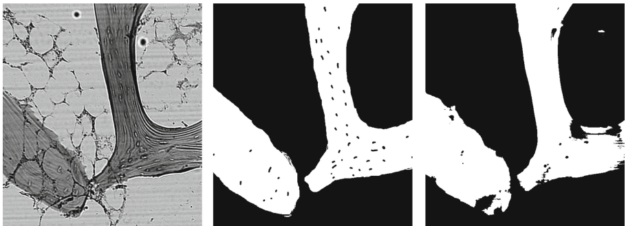
Fig. 5. Example results: original grayscale image (left), reference (middle), obtained segmentation (right)
