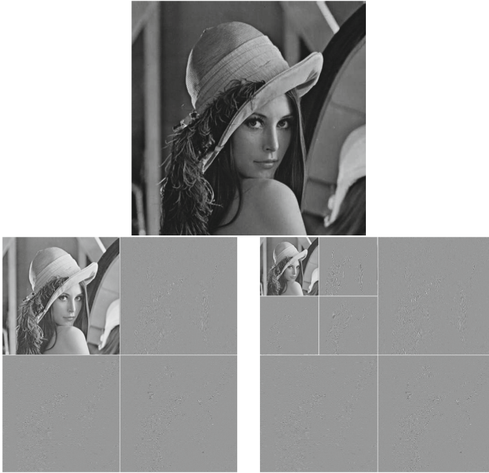
Fig. 1. Wavelet transform associated to Lena image for two decomposition levels. The size of the image is 512 by 512 pixels. The decomposition was performed using Daubechies wavelet with 12 vanishing moments. The approximation image corresponds to the subimage on the top left quarter. The other three subimages correspond to the projection of each approximation on a family of wavelets. We note that the main objects are relatively well preserved by each approximation image.
