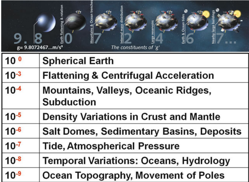
FIGURE 1.4. Illustration of the components of the gravity acceleration (ESA medialab, ESA communication production SP-1314).
