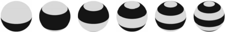
FIGURE 3.2. Zonal ( j = 0 ) spherical harmonics of different degrees 1, \dots, 6 (from left to right). The black and white color indicate the zones of different signs of the function, respectively.
