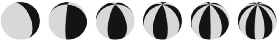
FIGURE 3.4. Sectorial ( k = \pm n ) spherical harmonics of different degrees. The black and white colors indicate the zones of different signs of the function, respectively.
