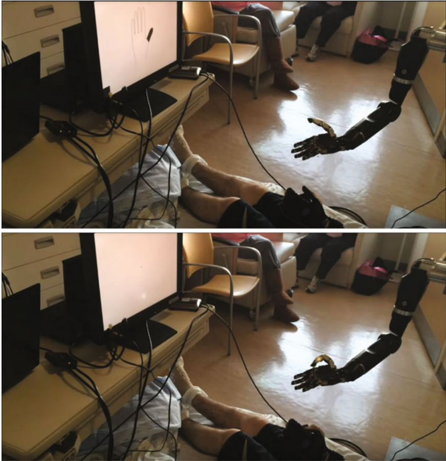
Fig. 4 Online control of individual finger movements. First a cue was presented on the screen highlighting the finger to be moved in black ( top ). The patient then flexed the highlighted finger 5 times. During the movement, the decoder classifies which finger is moving from the ECoG features and sends a command to the MPL to flex the same finger ( bottom )
