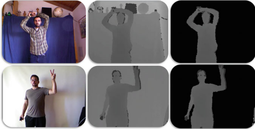
Fig. 10.2 Region of Interest detection. Left RGB video frames. Center depth frames. Right the detected ROI
