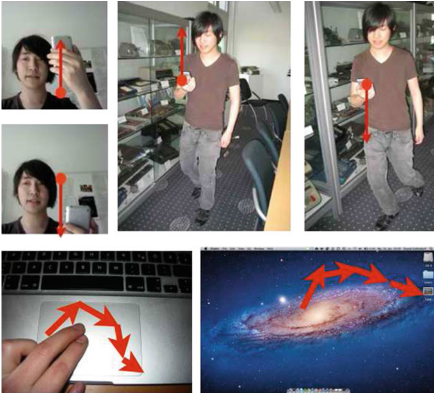
Fig. 4.1 Top a “shake-to-shuffle” gesture ( left ) can be confused with normal up-and-down movement while walking ( right ). Bottom a touchpad shortcut gesture ( left ) can be confused with normal cursor movement ( right )
