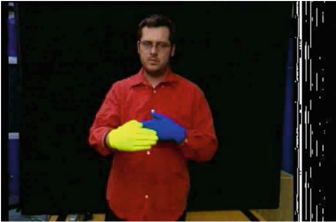
Fig. 3.13 Repetition of the appearance based sub-unit classifier vector. The band down the right hand side of the frame shows the sub-unit level classifier firing patterns for the last 288 frames, the vector for the most recent frame is at the bottom. The previous video during the 288 frames shows four repetitions of the sign ‘Box’
