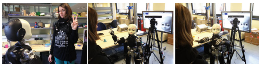
Fig. 10.10 The first two turns of a match. Left the human player performs the first gesture of the sequence. Center iCub recognized the gesture and imitates it. Right iCub adds a new random gesture to the sequence
