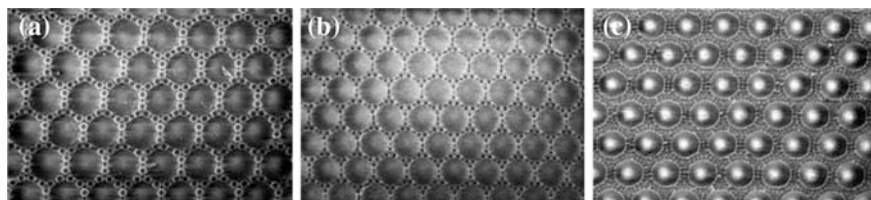
Fig. 2.8 SEM images showing binary microbead monolayers (Reproduced from Ref. [5] with kind permission of © 2003 Wiley-VCH)
