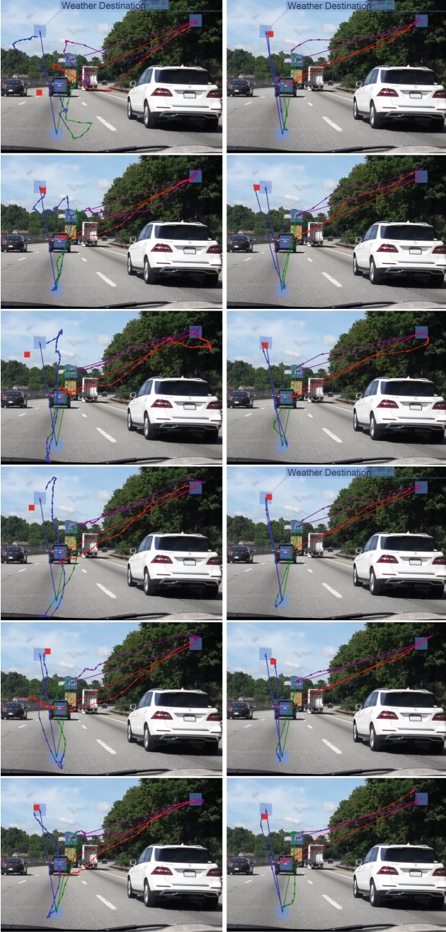
Fig. 13. Interactive HUD performance test. From top to bottom: user A to F, left: HUDConCap, right: touch pad. (Color figure online)
