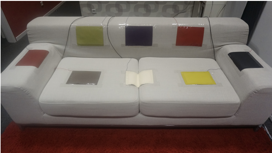
Fig. 1. Couch endowed with eight textile electrodes.
