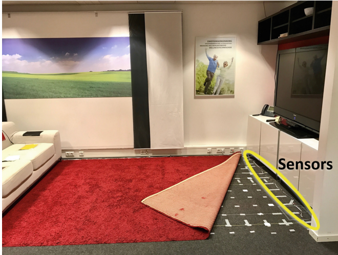
Fig. 5. Test setup in the living lab with electrode grid and sensors.
