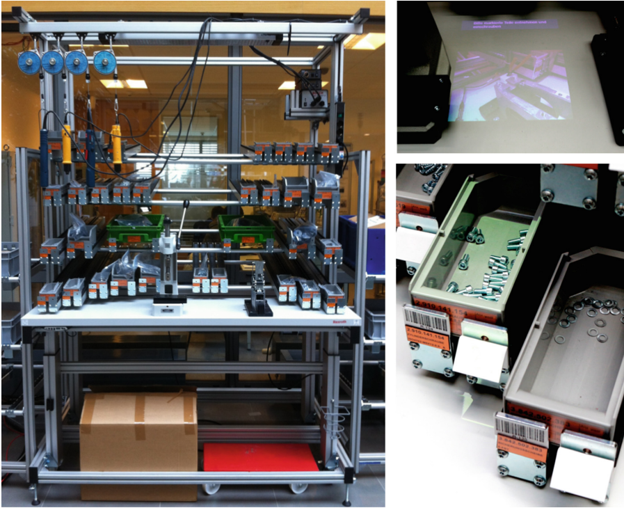
Fig. 1. Conventional manual assembly station (left) that was later equipped with assistive system with projection-based AR and intelligent hand tracking. Video-instructions are projected into the user’s workplace (right, top). In-situ projections highlight the boxes for picking with green light (right, bottom). (Color figure online)
