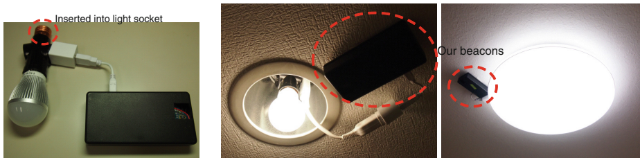
Fig. 1. Our developed beacon connected to an electric bulb.
