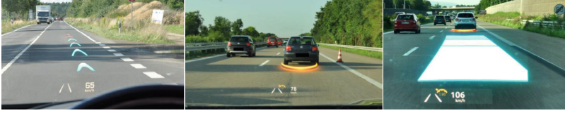
Fig. 1. Continental's augmented Head-Up Display prototype with different driving situations [11].
