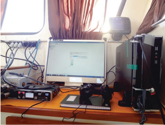
Fig. 5.3 Recording system composed by a fanless computer, a data acquisition board for frequencies higher than 192 kHz and an audio interface for frequencies below than 192 kHz. (Reproduced with permission of Franciele R. de Castro)
