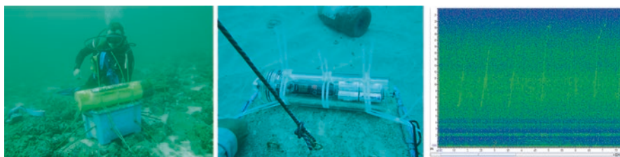
Fig. 12.14 Underwater acoustic recorders used to monitor the acoustic habitat of Cano and Murcielago Island in Costa Rica, both locations are protected areas used by humpback whales and dolphins. The last photograph shows spotted dolphin whistles recorder at 2 a.m. The project is funded and coordinated by Conservation International Costa Rica, and lead by Dr. May-Collado
