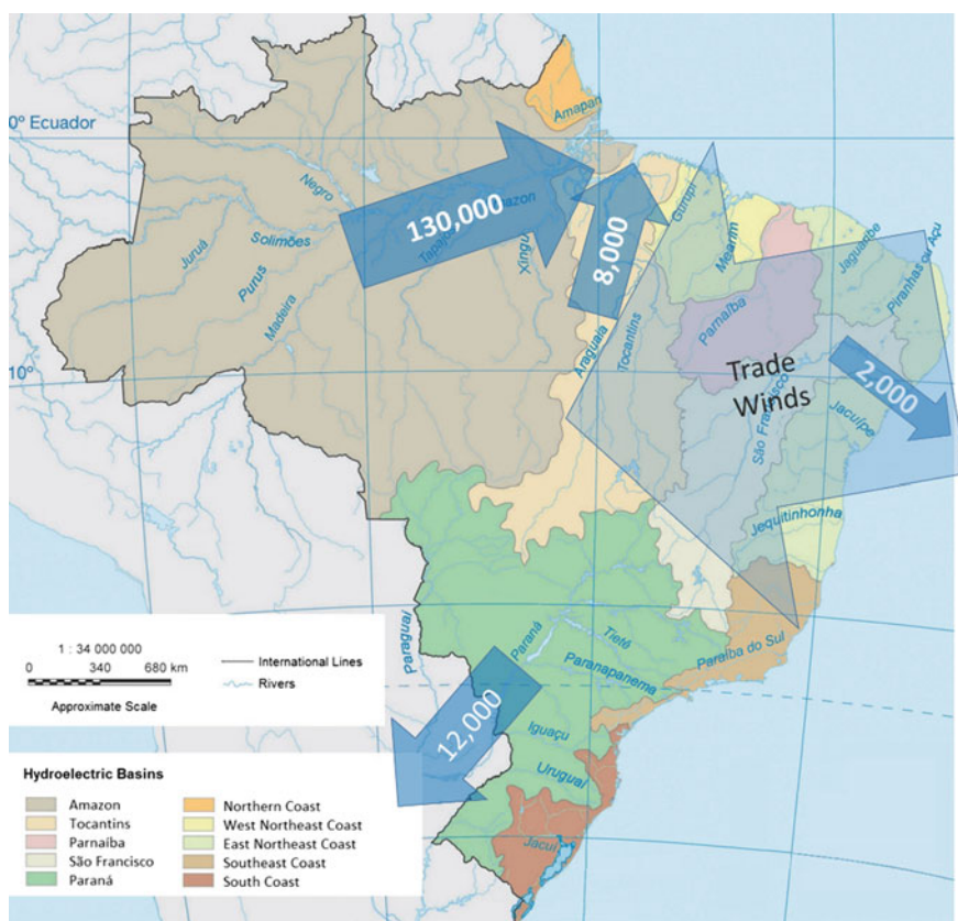
Fig. 11.5 Hydrological and climatic characteristics of major Brazil basins (numbers represent \text{m}^3/\text{s} ) (Operador do Sistema Nacional 2015)
