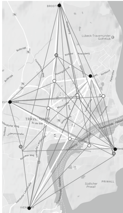
Fig. 7. Visualization of the allocations of all the demand points. A line means that the black marked demand point at the beginning of the line is assigned to the white marked practice located at the end of the line.
