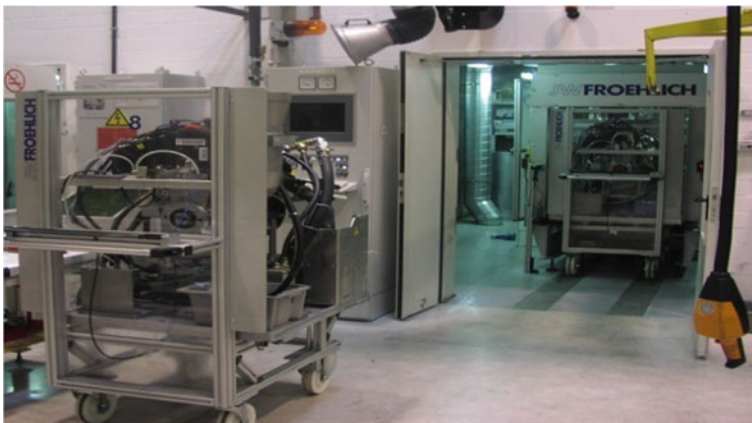
Fig. 21.2 Engines hot test machine (container type)
