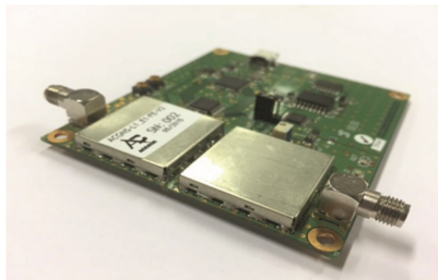
Fig. 4. AGC controlled sampler
