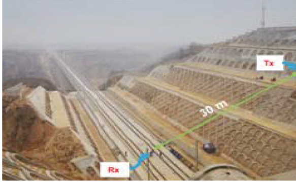
Fig. 2. Measurement setup. The receiver is over the track and the transmitter is 30 m away (on the right)
