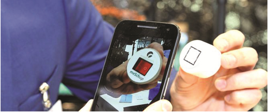
Fig. 6. Augmented Reality Interface extending a smart mobile lamp with a virtual on/off switch. Pressing the virtual switch on the screen instantly turns the lamp on or off.
