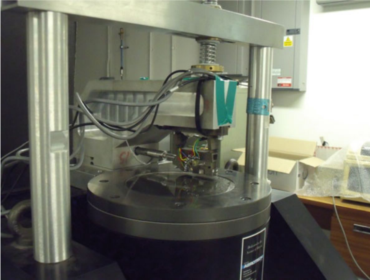
Fig. 12.27 Test rig with rotating disc and sensor and actuator pack
