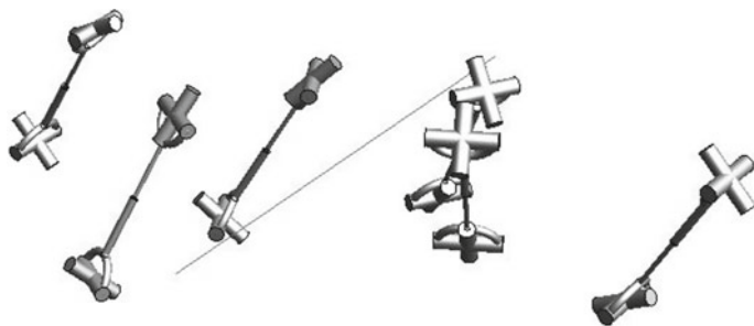
Fig. 4 A mobile 6UPU parallel mechanism constructed by reflecting three legs in the line shown. For clarity, the base and platform are not shown, the base connects the lower R joint of each leg and the platform joins the uppermost R joints
