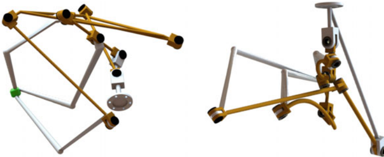
Fig. 6 Hand design for twist subspace, left ; hand design for approximate trajectory synthesis, right
