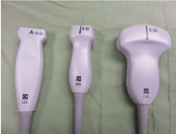
Fig. 6.1 Examples of different types of US probes. The probe to the left of the image is a linear (higher frequency) transducer useful for superficial applications and lung imaging. The probe in the center is a phased-array transducer useful for cardiac and deep “between-rib” applications. The probe to the right of the image is a curvilinear (lower-frequency) transducer useful for deeper (intra-abdominal) applications
