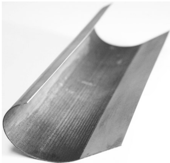
Fig. 10.20 Laser-bent steel sheet. Laser beam power 4.5 kW, beam velocity 1500 \text{ mm s}^{-1} , distance between irradiation lines 2 mm, 3 irradiations per line, carbon coating, sheet thickness 0.8 mm, material hot-rolled steel
