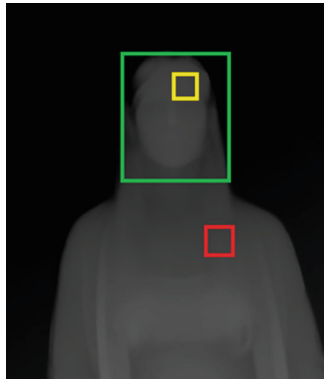
Fig. 3. Sampling process. Patches within the green rectangle, like the yellow one, are picked as positive samples. The ones outside, like the red one, are picked as negative. (Color figure online)
