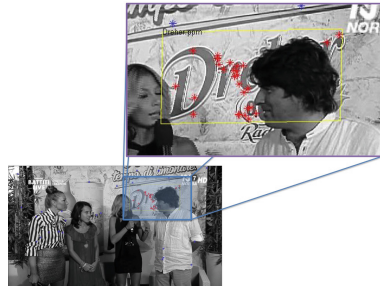
Fig. 8. Example of the the logo detection: the red stars represent inliers whereas the blue ones represent outliers (Color figure online)
