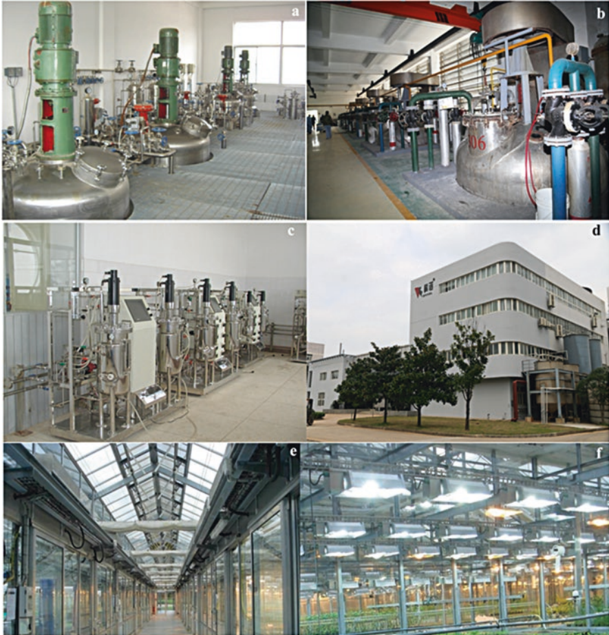
Fig. 12.5 Production of B. thuringiensis biopesticides by submerged fermentations in China. (a, b) Fermentors (Wuhan KeNuo Biotech, Inc.); (c), Seed fermentors (Wuhan KeNuo Biotech, Inc.); (d) Fermentation workshop (Wuhan KeNuo Biotech, Inc.); (e, f) Pesticide efficacy trials in the greenhouses (Hubei Kangxin Agro-industry Co., Ltd)
