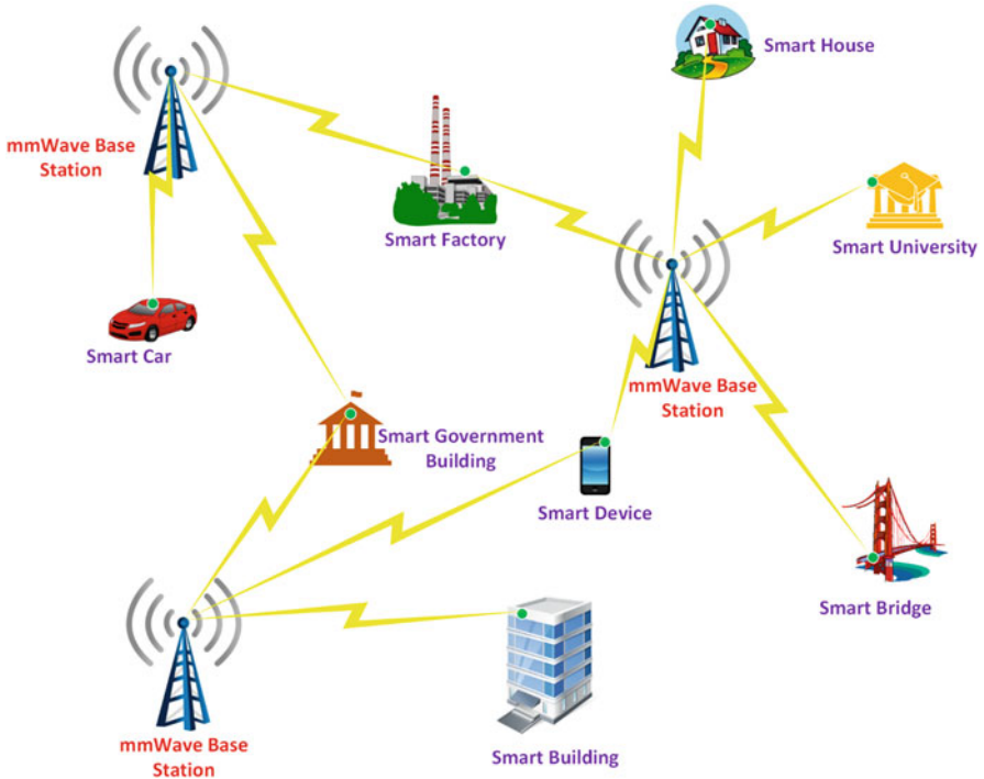
Fig. 1.5 Millimeter Wave (MmWave) assisted SWIPT/wireless power transfer (WPT) scheme. This shows how the mmWave assisted SWIPT enabling the universal access of 5G networks
