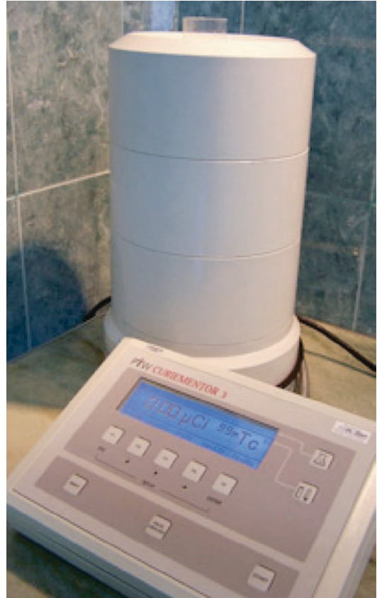
Fig. 6.9 The calibrator, adjusted for the use of Tc-99m
