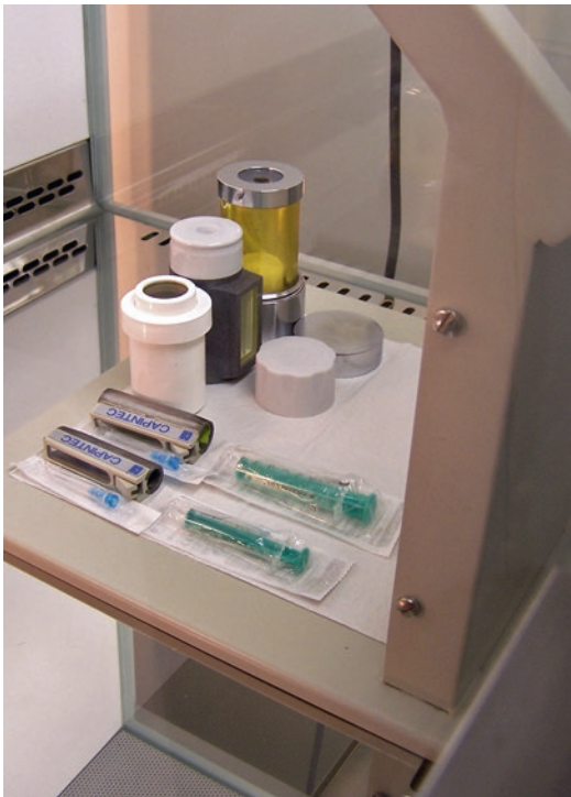
Fig. 6.5 Shielding for elution and injection preparation under sterile laminar flow
