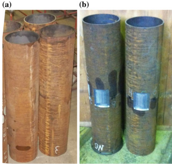
Fig. 15 a Blank pipes used for specimens; b VSDs machined on two specimens
