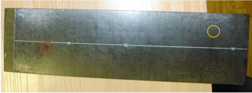
Fig. 2 Photo of a composite plate with orange and red rings showing the location of 5 and 9 J impact damage, respectively (color figure online)
