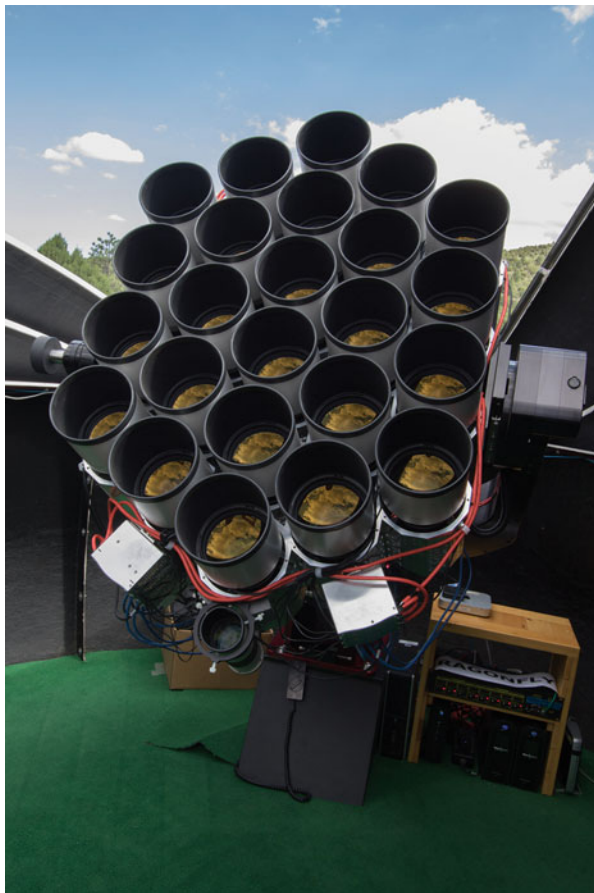
Fig. 10.2 One of the two 24-lens arrays comprising the 48-lens Dragonfly Telephoto Array. The lenses are co-aligned, and the full array is equivalent to a 1 m aperture f/0.39 refractor with a 2 \times 3 deg field of view. The arrays are housed in domes at the New Mexico Skies Observatories and operate as a single telescope slaved to the same robotic control system. The lenses are commercial 400 mm Canon USM IS II lenses that have superb (essentially diffraction-limited) optical quality. This particular lens has very low scatter on account of proprietary nanostructure coatings on key optical surfaces (see Abraham and van Dokkum 2014 for details). Each lens is affixed to a separate CCD camera, and both are controlled by a miniature computer attached to the back of each camera that runs bespoke camera and lens control software that we have made publicly available on a GitHub repository. In the latest incarnation of Dragonfly, each lens is self-configuring and is controlled by its own node.js JavaScript server in an “Internet of Things” configuration that provides a RESTful interface. Growing the array is done by simply bolting a new lens onto the array and plugging in network and power cables
